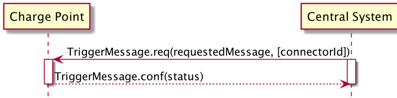
Figure 38. Sequence Diagram: Trigger Message
